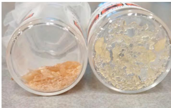
Polyhydroxyurethane with Tg-value above room temperature (left) and around room temperature (right)
